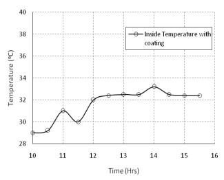
Fig. 5. Inside temperature with coating of reflective paint on the exterior surface
