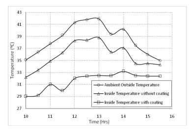
Fig. 6. Comparison of ambient temperature, inside temperature with and without coating
